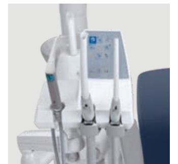
Assistant's module The module mounted on the double-articulated arm is height-adjustable and comes with three holders as standard. An optional 5-holder version is also available: this can be used to hold other instruments such as a video camera or T-LED light. The keypad incorporates controls that move the patient chair, switch on the operating light and operate the water-to-cup and cuspidor bowl rinse functions.
