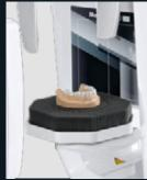
A specific protocol allows for tomographic scans of radiological templates, prostheses, models or impressions after they have been positioned on a special support.
